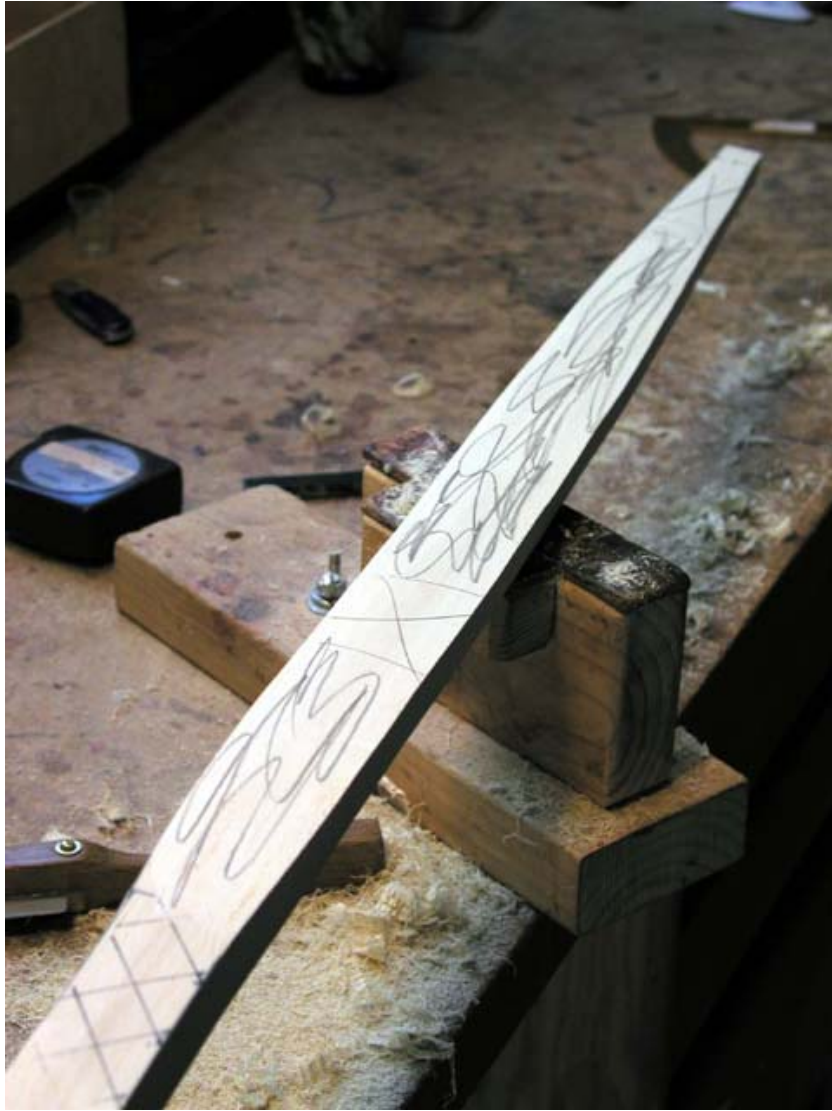
After a few iterations of wood removal the bow is bending a bit.
