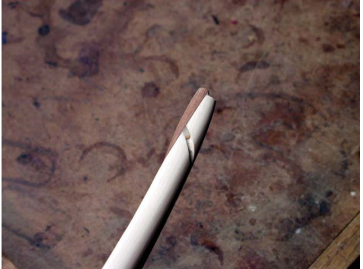
The groves are re-cut with a small rattail file.
