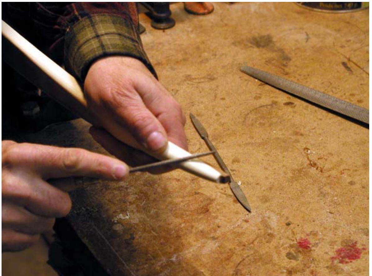
I make the groves meet at a point at the top of the overlay.
