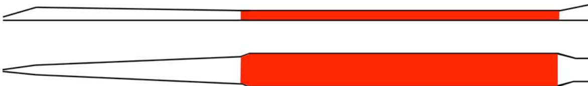
Figure 1: Side view profile of the Holmegaard limb (Not to scale). The parallel section is shaded. Note that the outer limb increases in thickness until near the tip then tapers down to a point. Compare the shaded area of the thickness profile with the plan view below it. The shaded areas indicate the area of parallel thickness.
